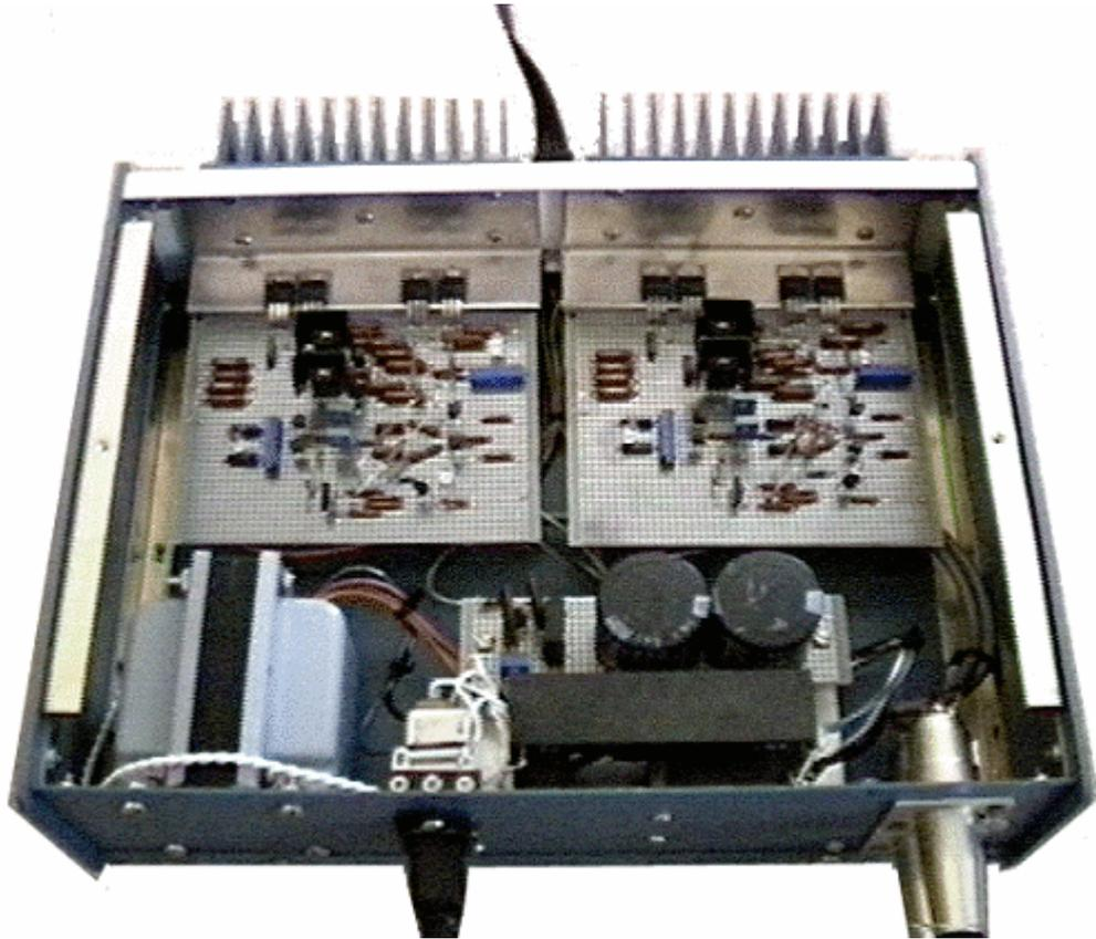
The enclosure is a Mod.U.Line by Precision Fabrication Technologies Inc. (part number 03-1209 and is available from Newark Electronics, probably Allied too. It measures 3" x 12" x 9".
