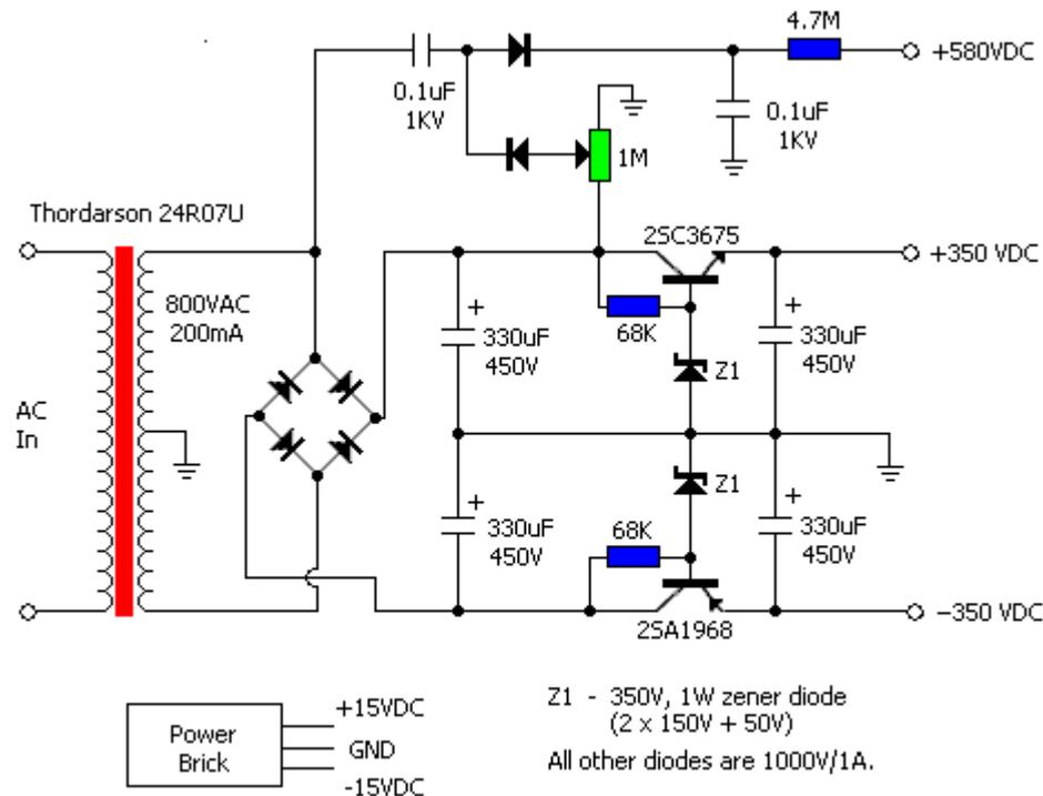
**Electrostatic Amplifier Power Supply**
