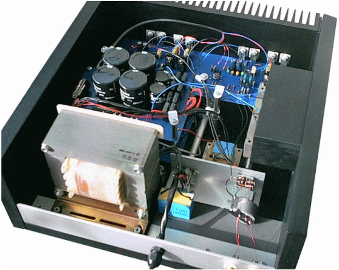
The two smaller transformers under the wooden cover are the 10H-chokes for the high voltage power supply. The little transformer on the bottom generates the bias-voltage. The oversized big-one is a special-made 250W transformer, from Experience-Electronics in germany. The electrolytics are from EPCOS (Siemens).
