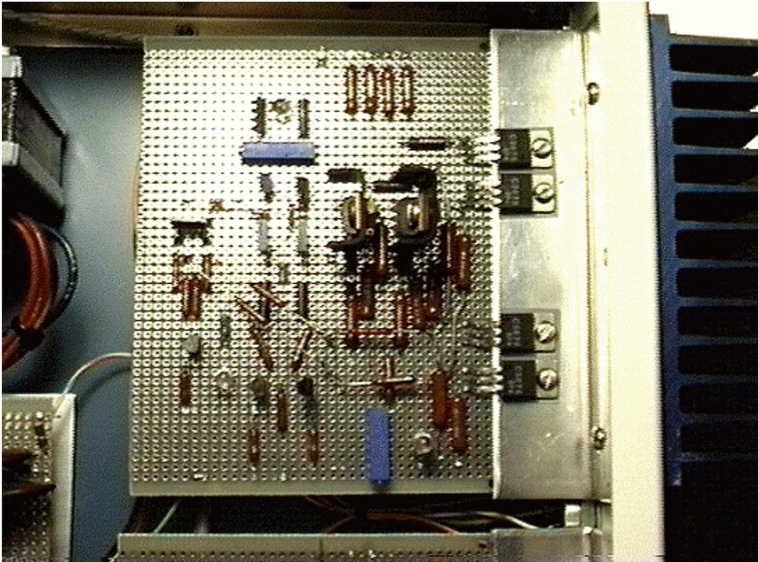
All 4 output transistors are mounted on one aluminum angle that bolts through the front panel to a heatsink. The mounting heatsink is 4" x 5" x 1/8" aluminum plate, punched and then bent along short axis. There are 4 holes that hold the transistors to the angle, and 5 holes that bolt the angle to the heatsink. The blue-finned heatsinks I found on some old power supplies. I used them because they were big enough and pretty at the same time. The 2 2SC3675 drivers have small standup heatsinks.
