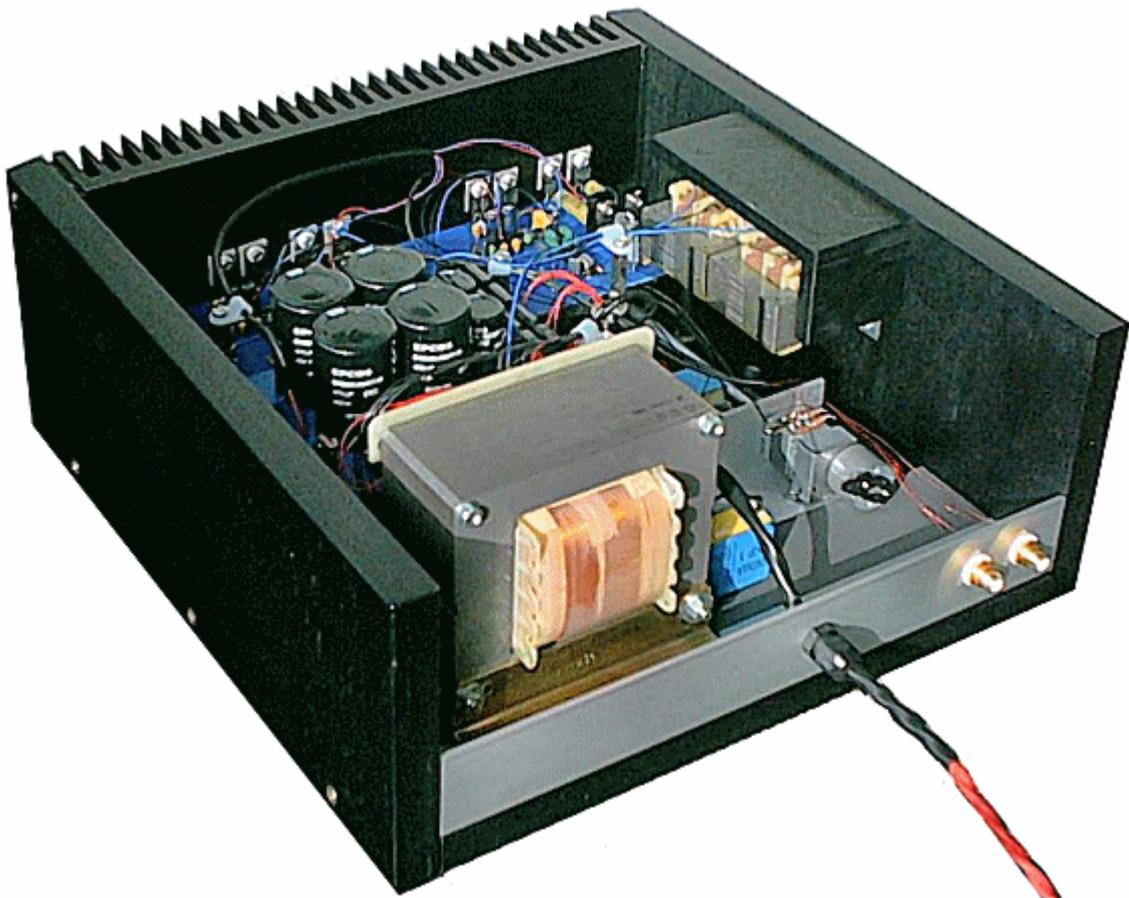
The Cabinet is a very simple construction, with the advantage of ease changing components or parts. There is only a wooden base with two side-panels. The front is the large heatsink together with an aluminium-angle. A suitable top-cover is under construction. The whole construction could be made way smaller, all parts on one pcb, with a smaller toroid-transformer, and all built in a industrial case, but for my own usage, it's ok.
